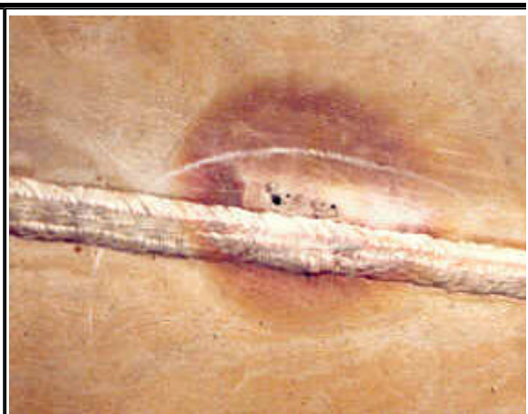
Fig 4: Detail of a pit near the bottom weld
